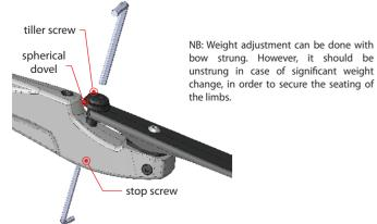
To make adjustment easier, groooves are engraved on the screws. Following pictures illustrate the 3 positions identified, accordingly to groove alignment with the edge of the riser (alignment should be obtained compared to the «highest» edge of the riser).
