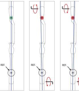
the string is aligned with both of the tiller bushings -> no action required at this step, move up to step 2
